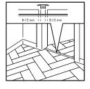
In a glued installation you have no length and width restrictions. An expansion gap of 8 mm around the perimeter of the room is still obligated but a T moulding in the doorways is not necessary anymore. Constructional dilatation joints of the building and floor heating joints in screed should be transferred on the floor with a flexible joint or a profile.
